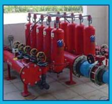
Compact automatically controlled systems for proportioning fertilisers, acids and phytosanitary products.
